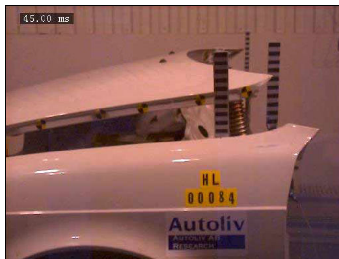
Figure 22 - Bonnet with protection system in activated, lifted position,
